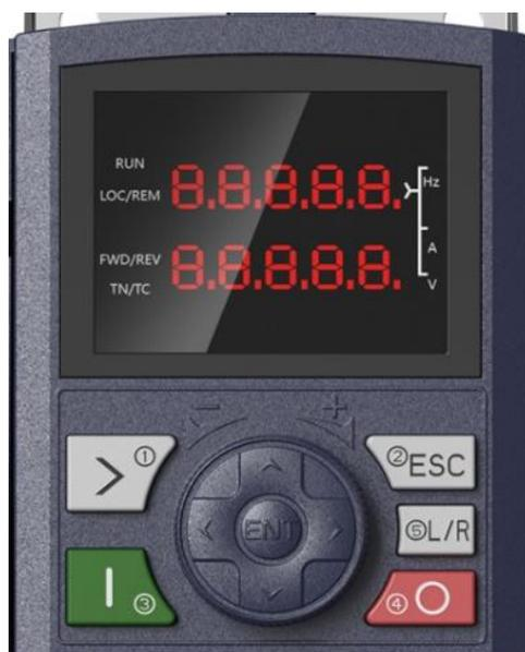
Schematic diagram of operation panel
